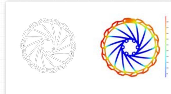
Heat transfer within the design concepts was studied extensively using advanced engineering software. The relationships between convection, radiation, surface area and weight were used to determine the optimal design to maximize heat dissipation and strength while minimizing weight.
